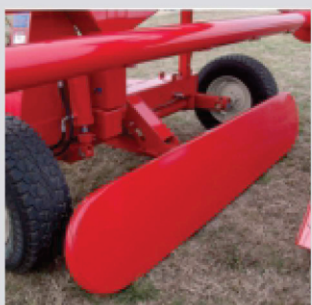
Grain pusher pan improves "end of bag" clean up & performance in tough grain conditions.
